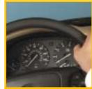
Changing the gellant from lithium soap to a superslippery PTFE solved a stick/slip problem in a telescoping steering column. The PTFE added just enough lubricity to make up for a lack of oil at the interface at start-up.
