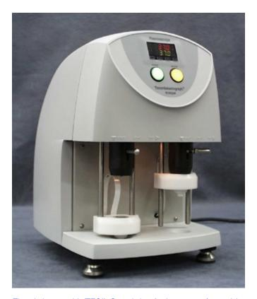
Thrombelastograph<sup>®</sup> (TEG<sup>®</sup>) Coagulation Analyzer, manufactured by Haemoscope Corporation of Skokie, Ill., tracks the shear elasticity of a clot and its ability to arrest bleeding — in real-time, during a medical procedure. It relies of two greases by Nye Lubricants, one in the gear motor and one where mating parts slide on the frame.
