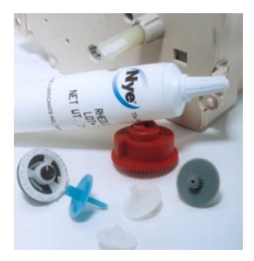
Mallory Controls of Indianapolis, Ind., chose a low-viscosity, synthetic hydrocarbon base oil combined with a lithium-soap thickener and special lubricity and adherence additives to meet the low-temp, low startup torque requirements of plastic gears in its Model 620 appliance timer. The grease was custom-designed by Nye Lubricants, Inc.
