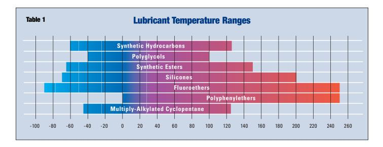
esters, at 175°C; silicones, at 200°C; and PFPEs at 250°C or higher. Most synthetics also take the cold. Polyglycols stay lubricious at -40°C; synthetic hydrocarbons, at -60°C; synthetic esters, at -65°C; silicones, at -70°C; and some PFPEs, at -90°C (*See Table 1, "Lubricant Temperature Ranges"*)
