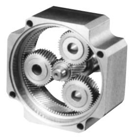
In Bayside Control Group's precision gear set even a film of lubricant can potentially be thick enough to cause a positioning error. A very light thixotropic grease not only passed rigorous life tests, it lowered internal temperatures by five degrees.
