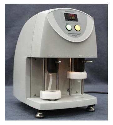
**Figure 4** Thrombelastograph<sup>®</sup> (TEG<sup>®</sup>) Coagulation Analyzer, manufactured by Haemoscope Corporation of Skokie, III., tracks the shear elasticity of a clot and its ability to arrest bleeding — in real-time, during a medical procedure. It relies of two greases by Nye Lubricants, one in the gear motor (see below) and one where mating parts slide on the frame.
