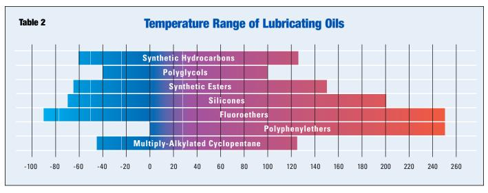
Synthetic oils offer a broader operating temperature range than petroleum lubricants, whose temperature limits range from about -18°C to +100°C.
