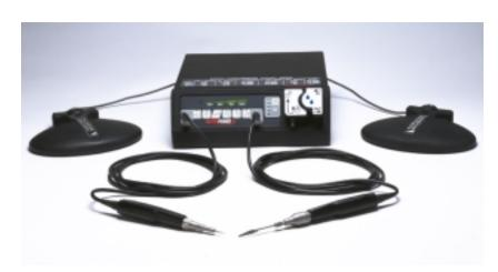
**Figure 3** A modular surgical handpiece system by OsteoMed Corporation is used for the dissection and drilling of small bones. A filtered, fortified synthetic hydrocarbon oil by Nye Lubricants is recommended prior to autoclaving to flush and lubricate bearings in the system's 11 saw and drill attachments. High-speed dental handpieces also use synthetic hydrocarbon oils in the turbine bearings. Typically, the bearings are re-lubricated with oil and placed in an autoclave after each use.
