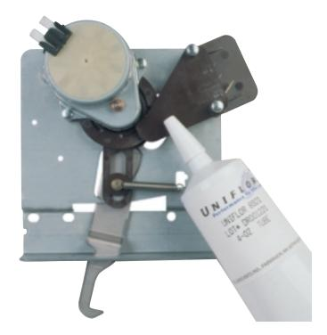
**Figure 1** Kingston's new low-profile, motorized range lock relies on thermo-plastic parts lubricated with a PFPE/PTFE grease to survive oven cleaning-cycle temperatures in excess of 232°C. Its Class N motor also uses a PFPE/PTFE grease.
