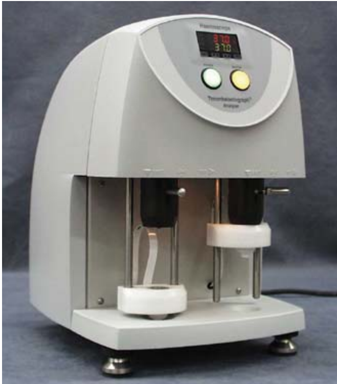
Figure 4 Thrombelastograph® (TEG®) Coagulation Analyzer, manufactured by Haemoscope Corporation of Skokie, Ill., tracks the shear elasticity of a clot and its ability to arrest bleeding — in real-time, during a medical procedure. It relies on two greases by Nye Lubricants, one in the gear motor (see right) and one where mating parts slide on the frame.
