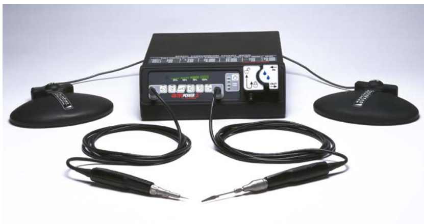
Figure 3 A modular surgical handpiece system by OsteoMed Corporation is used for the dissection and drilling of small bones. A filtered, fortified synthetic hydrocarbon oil by Nye Lubricants is recommended prior to autoclaving to flush and lubricate bearings in the system's 11 saw and drill attachments. High-speed dental handpieces also use synthetic hydrocarbon oils in the turbine bearings. Typically, the bearings are re-lubricated with oil and placed in an autoclave after each use.
