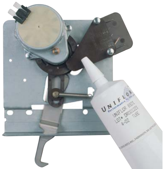
Figure 1 Kingston’s new low-profile, motorized range lock relies on thermo-plastic parts lubricated with a PFPE/PTFE grease to survive oven cleaning-cycle temperatures in excess of 232°C. Its Class N motor also uses a PFPE/PTFE grease.
