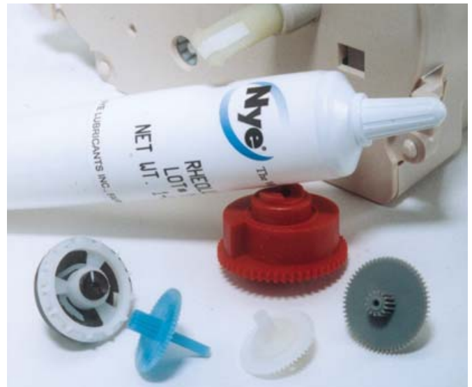
Figure 2 Plastic gears in Mallory Controls’ Model 620, a timer for commercial laundry, laboratory cleaning equipment, dairy equipment, and domestic clothes washers and dishwashers, use a NLGI Grade 2 synthetic hydrocarbon grease with special lubricity and adherence additives. Mallory reported that the grease reduced gear tooth wear, dampened acoustic noise, and substantially increased timing cycles.
